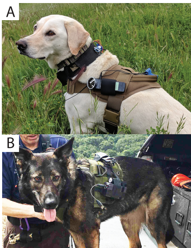
Figure 2. Search and rescue dog wearing research harnesses. (a) Audio recorder, microphone collar, and tilt switch (blue chip attached to collar) are shown. (b) Data logger for GPS and tilt switch.
